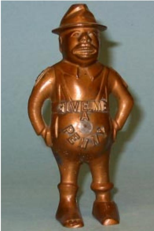
**Photo 1.** Brass working pattern for a "Give Me a Penny (screw)" bank, M-166.
