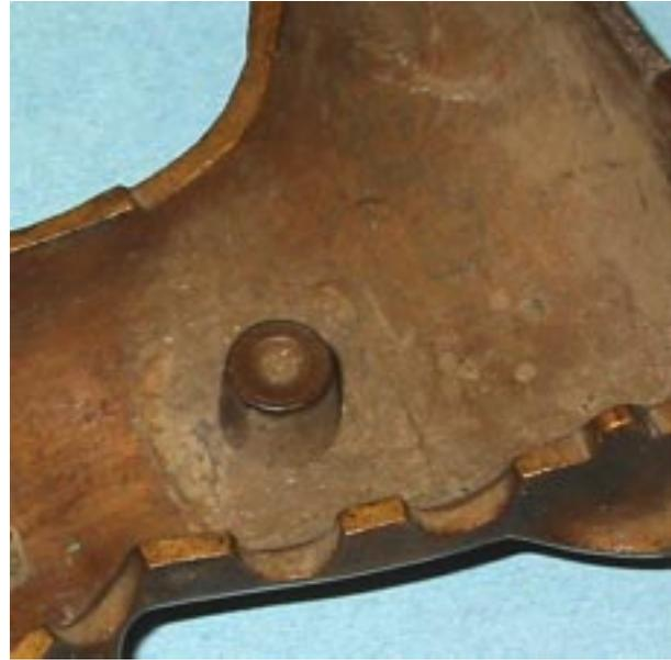
**Photo 4.** Close-up of the inner surface of the left side of the pattern and the post or "boss." The area around the post is coated with solder. Beyond the left edge of the photo is a pattern number, "989." This number also is stamped in the right half.
