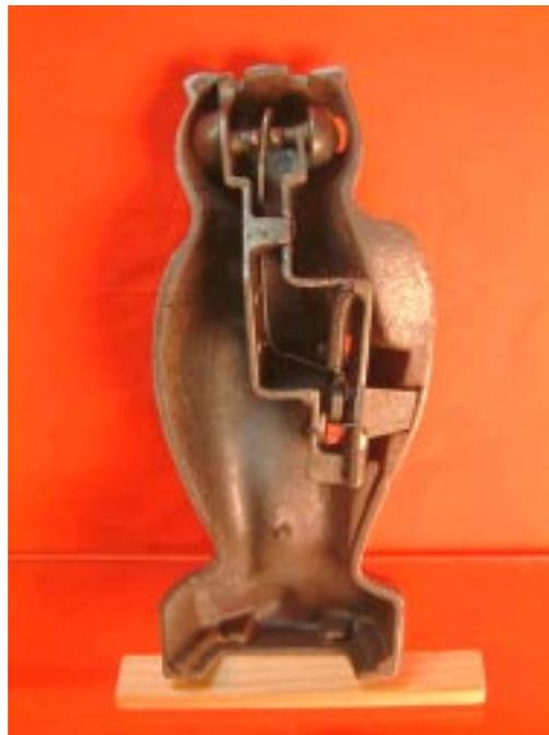
**Illustration 20.** The front half and the internal mechanism of an "Owl, Slot in Book" bank.
