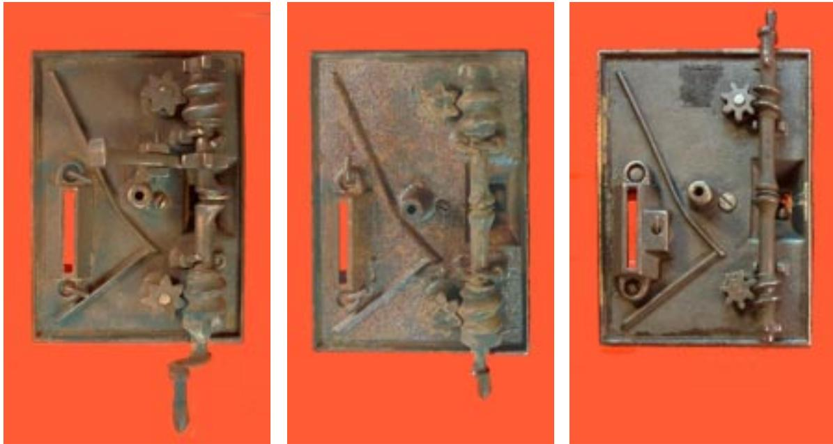
**Illustration 21.** Three different internal mechanisms used in the "Organ Bank, Cat and Dog" banks by Kyser & Rex Co.
