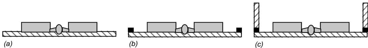
**Figure 3.** (a) The pattern tree placed cope-side down on the follow board. In (b) a spacer frame has been placed on the follow board, and in (c) the drag half of the flask has been added. (The central gate is shown penetrating the top surface of the follow board, but this was not necessarily the case and is ignored in the explanation.)
