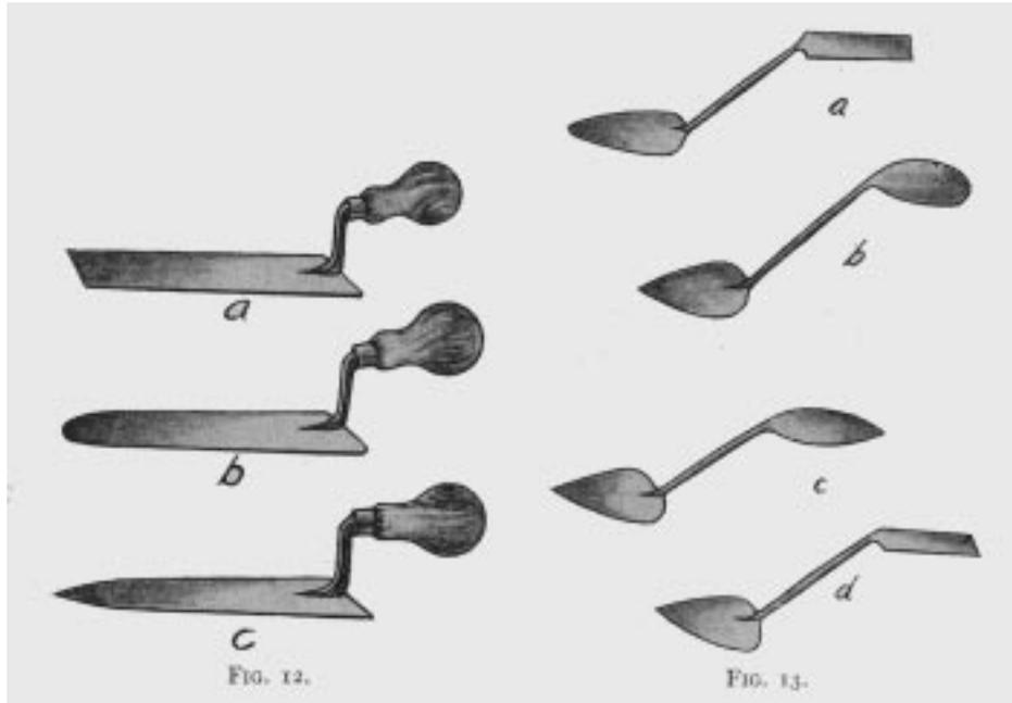
**Figure 6.** Examples of Molders' trowels and slicks from "A Text-Book of Elementary Foundry Practice."<sup>4</sup>
