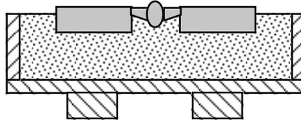
**Figure 2.** The drag half of a green-sand mold.
