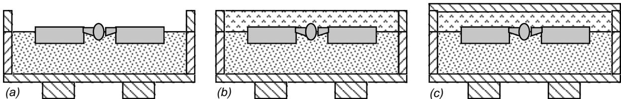
**Figure 7.** (a) The frame for the composition match has been added and in (b) the frame has been filled with the sand composition, rammed, and trimmed. In (c) a bottom board has been added and nailed or screwed to the frame.
