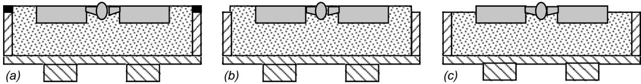
**Figure 5.** (a) The wood follow board has been removed, and in (b) the spacer frame also as been removed. In (c) the joint has been cut; molding sand has been removed down to the parting line of the mold.
