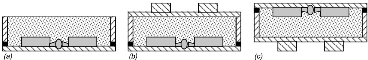
**Figure 4.** (a) The drag has been filled with molding sand, rammed and trimmed. In (b) a bottom board has been added, and in (c) the mold has been rolled over.
