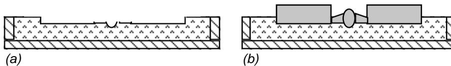
**Figure 1.** (a) Cross section of a match mold and (b) the match mold with its complementary pattern tree inserted.
