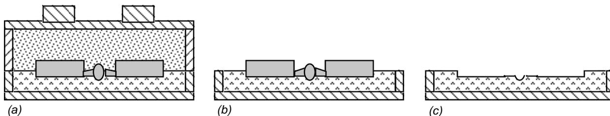
**Figure 8.** (a) The mold was rolled over and (b) the drag lifted off. (c) The finished composition match. After the sand composition has hardened the new composition match is ready for use. Note Figure 8(c) is identical to Figure 1(a).
