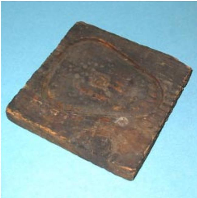
**Photo 1.** Jig for assembling the "Flat Iron Building" bank.
