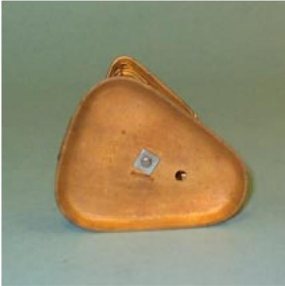
**Photo 2 .** Underside of the base. Note the ridge just below the square nut. This prevents the nut from turning when the bolt is tightened.
